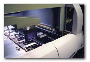
The LH SlideStainer's robotic arm retrieves the basket and moves it into the staining module for automated fixing, staining and drying.
